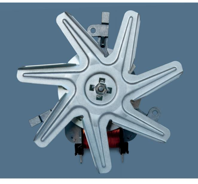
Pyrolytic ovens are a real boon to cleanliness. Though they relieve the housewife or househusband of messy work, the hot-air blower does not get any relief at all. It must withstand temperatures up to 500 °C over a lengthy period of 1-2 hours without any decrease in output or function.
