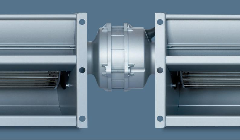
In large tangential blowers – such as those used for underfloor convection heating or air curtains – our newly developed size 43 motor with leading edge GreenTech EC technology is used. The three-core internal rotor motor features outstandingly high efficiency and virtually silent operation. In addition, operating electronics that are tuned exactly to the motor offer individual and precision control options.
