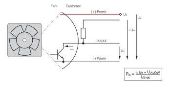
All voltages measured to ground. External load resistor  ${\rm R}_a$  from  ${\rm U}_A$  to  ${\rm U}_{BA}$  required.
