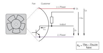
All voltages measured to ground. External load resistor  $\rm R_{A}$  from  $\rm U_{A}$  to  $\rm ~U_{BA}$  required.
