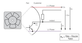
All voltages measured to ground. External load resistor  $R_a$  from  $U_A$  to  $U_{BA}$  required. With VARIOFANs with external temperature sensor for controlling the motor speed, the NTC sensor is not included in the scope of delivery. Temperature sensor LZ 370, see Accessories.
