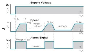
$t_2 = \mbox{Alarm signal suppression during start-up} \\ ^* \ n < \mbox{speed limit } n_G \mbox{ by braking or locking}.$
