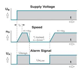
$\begin{aligned} &t_2 = \text{Alarm signal suppression during start-up.} \\ &\star n < \text{Speed limit } n_G \text{ by braking or locking.} \end{aligned}$
