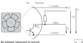
All voltages measured to ground. External load resistor  $\rm R_{a}$  /  $\rm U_{S}$  /  $\rm U_{BS}$  required.
