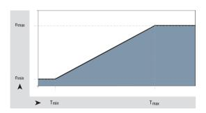
$$\begin{array}{l} n_{min} \, \approx \, 800 \, ^{1} /_{min} \, n_{max} \, \, \, \text{model-dependent} \\ T_{min} \, \approx \, 5 \, ^{\circ}\text{C} \, \qquad T_{max} \, \leq \, 85 \, ^{\circ}\text{C}, \, \text{model-dependent} \end{array}$$
