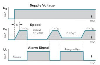
$t_2 = Alarm signal suppression during start-up.$
