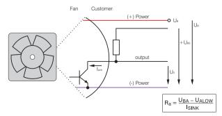
All voltages measured to ground External load resistor Ra from  $\rm U_{\mbox{\footnotesize A}}$  to  $\rm U_{\mbox{\footnotesize BA}}$  required.
