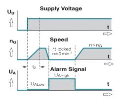
$\begin{array}{l} t_2 = \text{Alarm signal suppression during start-up} \\ ^* n < \text{Speed limit } n_G \text{ by braking or locking} \end{array}$
