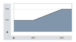
$$\begin{array}{ll} n_{min} \approx & 1/_2 \; n_{max} \\ T_{min} \approx & 30 \; ^{\circ}\text{C}; \, T_{max} = 50 \; ^{\circ}\text{C} \end{array}$$
