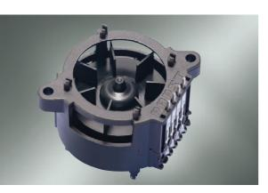
Small sensor blower for active ventilation of temperature sensors used for climate control in cars. The active ventilation avoids mismeasurements due to irradiation of various heat sources. Significant reduced overall size due to the new motor technique of an external rotor motor on pinch pole basis.
