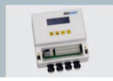
Stand-alone control device for refrigeration and air-conditioning technology in conjunction with the corresponding sensors. Using the controlled 0–10 V output or RS485 MODBUS RTU connection, ebm-papst fans with a corresponding input can be triggered. The function includes multifunctional pressure and temperature control as well as display and entry of various parameters. The integrated LCD display provides easy operation across multiple levels.
