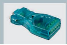
This interface converter permits bi-directional connection of RS232 devices (laptop or PDA) with bus-compatible devices (electronic commutation units with RS485 interface). The power supply is from the RS232 output of the laptop or PDA.
